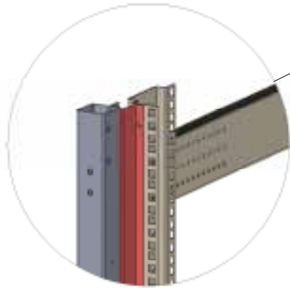
W=600 skirting panel for blocking cold air loss-vertical at 19" rails
